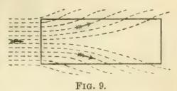
Slip of air over a short-span plane.
